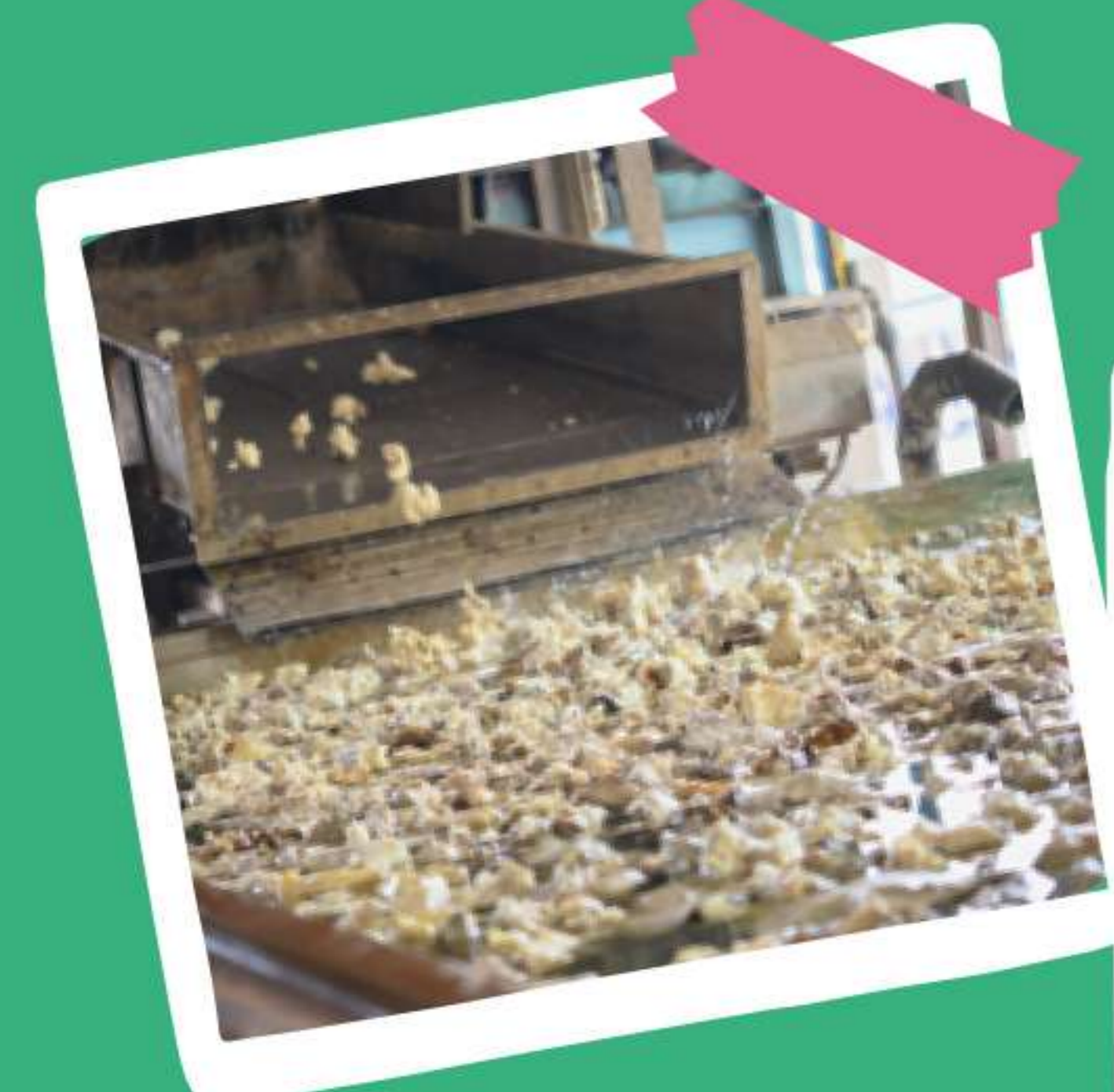
As it dries, the latex forms chunks which are washed, spread out, heated, compressed...
